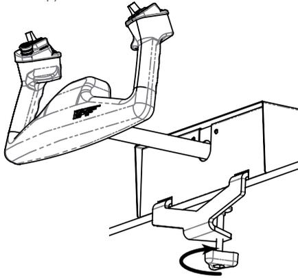
**2.2.** In case you have specific support, screw the YOKO+ with the clamping knobs (D). You can find the CUT-OUT measures in DXF format in our DOWNLOADS YOKO+ section: <https://www.virtual-fly.com/en/downloads>
